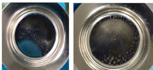
Fig. 2. Status of Pt crucible before (left)/after (right) \text{LiBO}_2 fusion of Actinide resin.
