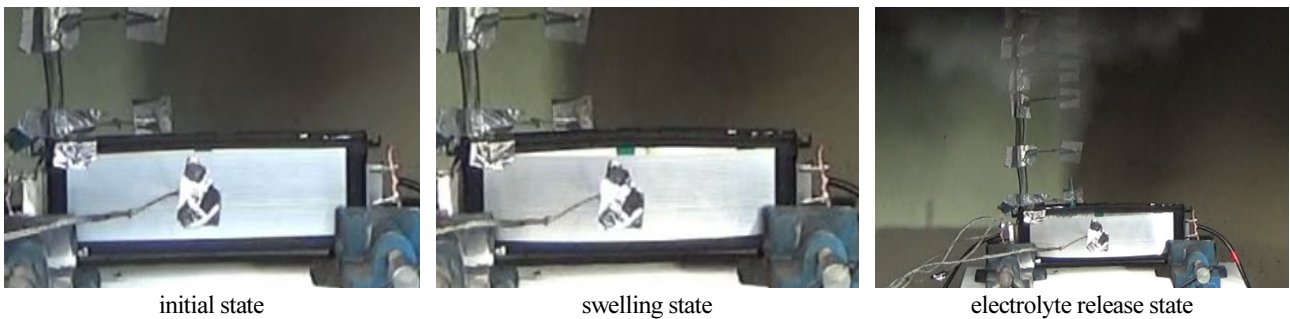
Fig. 6. Experimental results of lithium polymer battery overcharging test.
