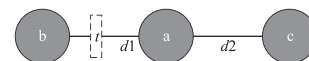
Fig. 4. The assessment of association value in both cases. Assume that the distance between protection element a and b is d_1 , the distance between a and c is d_2 . The task passed through the obstacle requires t minutes. The total time moved from element a to b is d_1/v + t .
