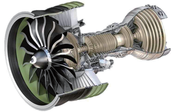
Fig. 5 General Electric GEnx Engine (Soft-wall Containment)
