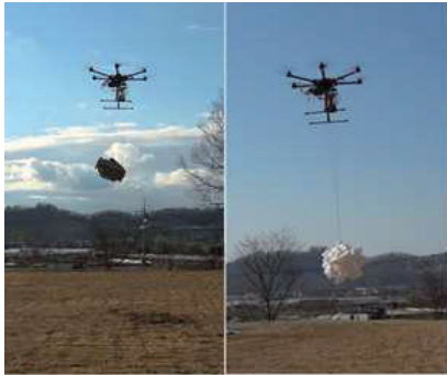
Fig. 12 Field test of the drone with capturing device
