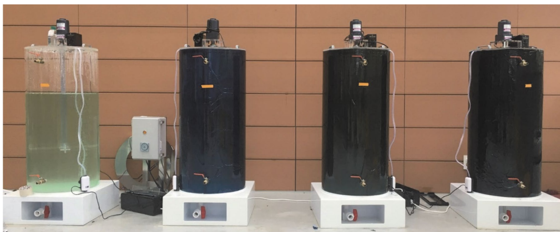
Fig. 1. Large-scale cultivation system in this study (Control, blue, green and blue/green groups in order, from the left).
