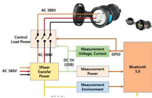
Fig. 2. Smart Plug Hardware Configuration.
