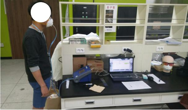
Fig. 3. The actual experiment of quantitative fit testing.
