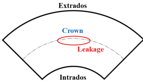
Fig. 3 Elbow specimen with leakage
