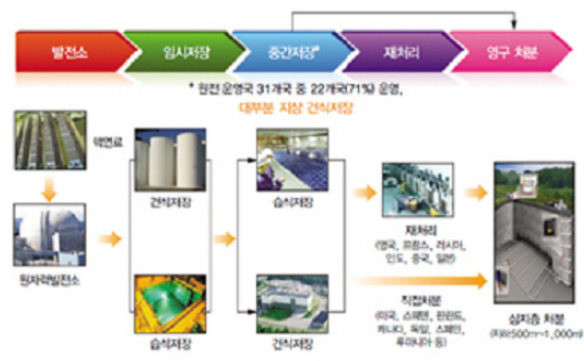
Fig. 1 Nuclear Spent Fuel Management Process
