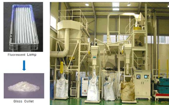
**Fig. 3.** Fluorescent lamp recycling facility (company of C).
