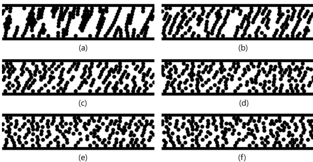
Fig. 6. Configuration of volume fraction \phi = 0.3 suspension at E = 1.0 kV/mm and \gamma = 10 (a) Mn = 0.0031 , (b) Mn = 0.031 , (c) Mn = 0.062 , (d) Mn = 0.16 , (e) Mn = 0.31 , (f) Mn = 3.1 .
