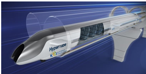
Fig. 1. Concept of the capsule train[1]
