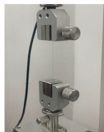
Fig. 1. Experimental apparatus for tensile strength of hair
