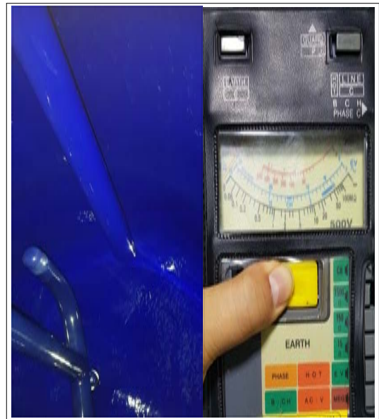
Fig. 2. Earthing Resistance (Glass Lined).
