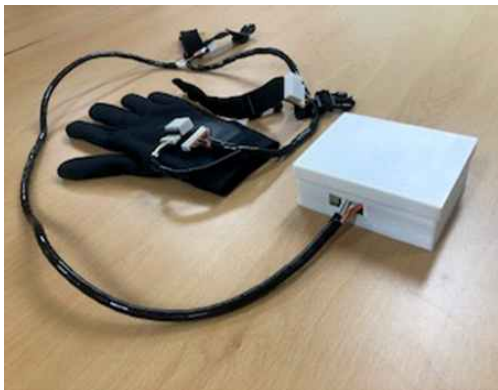
Fig. 5. An implemented glove and a control box
