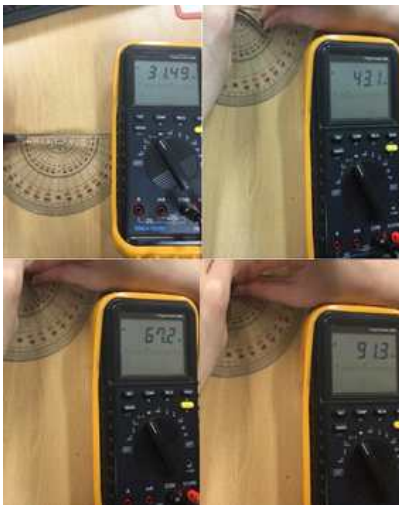
Fig. 3. Measurement of a flex sensor resistance according to its bending
