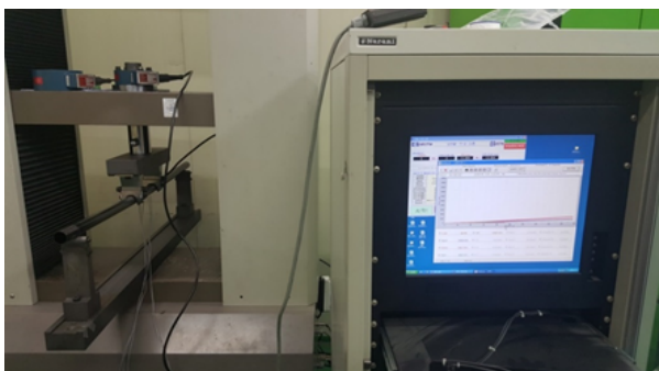
Fig. 5. Test setup for four-point bending test
