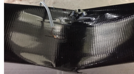
Fig. 7. Buckling failure mode (ovalization) of circular spar
