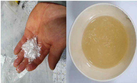
Figure 5. Chopped roving fiber and resin mixed putty
