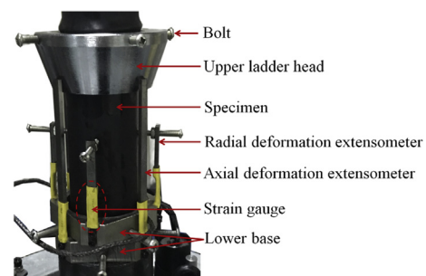
Fig. 2. Deformation sensor for axial and radial displacement measurements.
