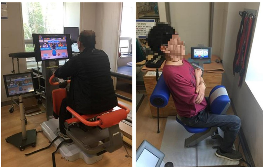
Figure 2. Trunk control robot intervention used 3DBT-33 (Man & Tel Co., Ltd, Gumi, Korea) (A), Trunk extension intervention used Abdomen/Back Extension Rehab 5310 (HUR, Helsinki, Finland) (B), and Informed consent was obtained from the patient for the publication of their image.
