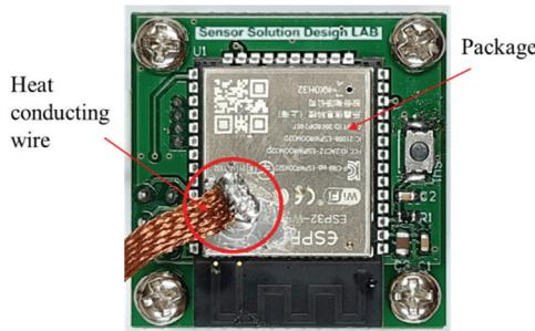
**Fig. 6.** Electronic components directly connected to the cold side cooling fins with heat conducting wire.
