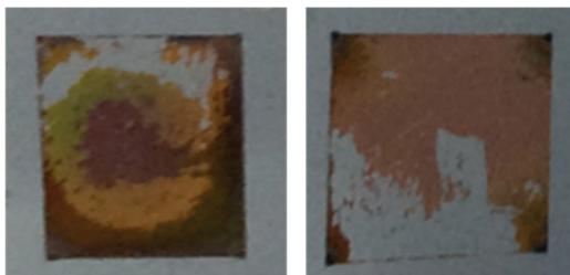
**Fig. 2.** Photos of CuO film peeling-off from wafer substrate after annealing (10, 20 mTorr).
