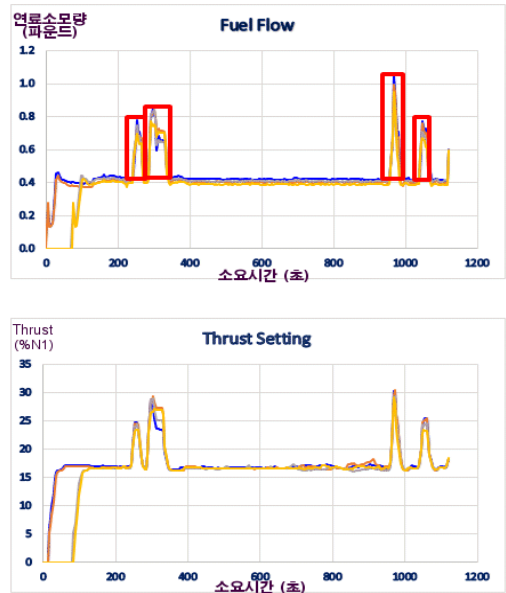
Fig. 4. Aircraft taxi fuel consumption prediction model(2) - Case #2
