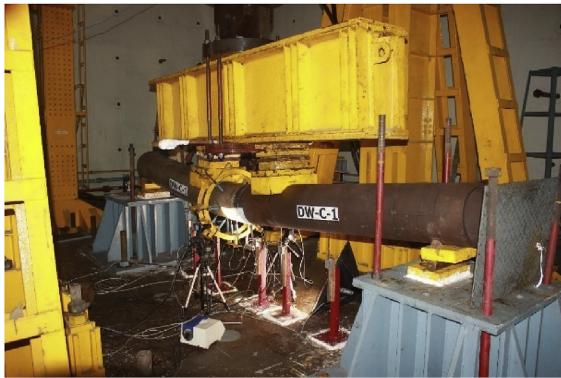
Fig. 5. Final deflected shape of the pipe.
