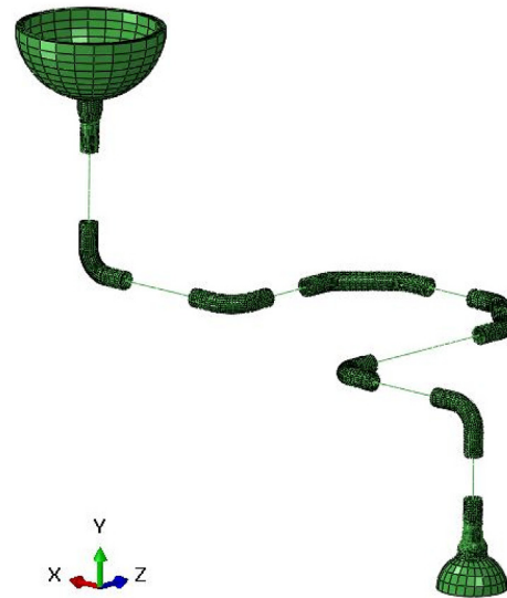
Fig. 4. Hybrid FE model of the pressurizer surge line.
