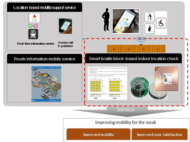
Fig. 1 Overview of Positioning System in Railway Station based on Smart Braille Block.
