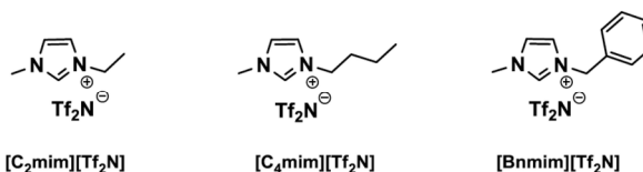
Fig. 5. [Rmim][Tf 2 N] ionic liquids (ILs) utilized to form polyimide-ionene + IL composites (Reproduced with permission from O'Harra et al. , 22).
