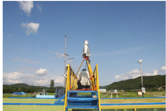
Fig. 4. 3D scanning for measuring scour depth, length, and volume.
