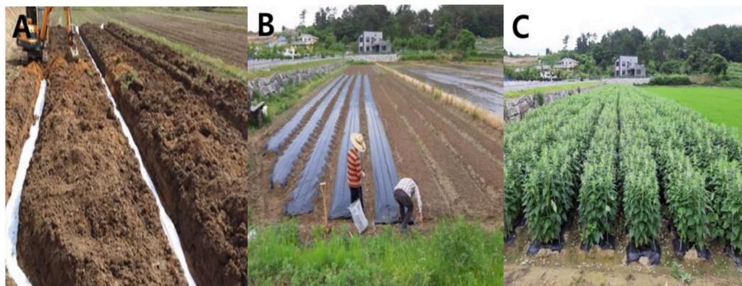
Fig. 1. Plant growth experiment according to the existence of drainage system. (A) Application the Non-excavated subsurface drainage system (Type 3) in Gae-san, (B) Set up the growth experiments in Gae-san, (C) Performed Sesamum indicum growth experiments.
