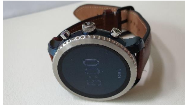
Fig. 9. Multi-function side buttons on Fossil Q Explorist.
