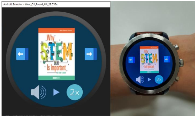
Fig. 10. Implementation of the WABA on Android emulator and a commercial smartwatch.
