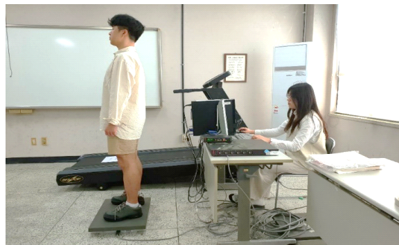
<Figure 3> The Subject and Experimenter Measuring Center of Pressure(COP)
