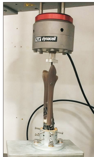
Figure 2. Testing machine to apply repetitive load to sawbone model.
