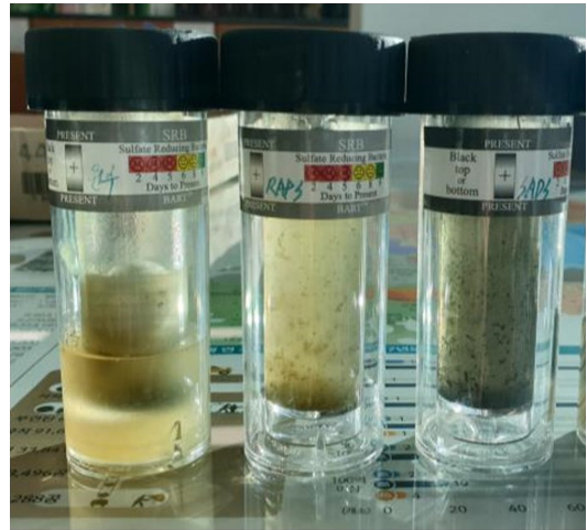
Fig. 11. SRB analysis results of the mine water and effluent of RAPS and SAPS using SRB test kits, showing that SRB is the most active in SAPS.
