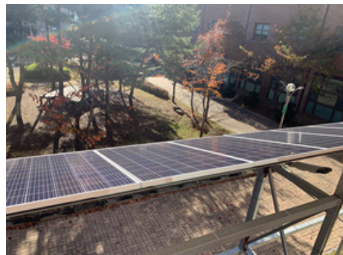
Fig. 8. Solar panel for irradiation data gathering
