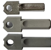
Fig. 11. Ball Safety Pin (finished part, green part, brown part)
