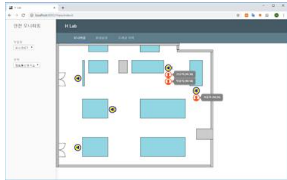
[Figure 11] Worker location monitoring screen
