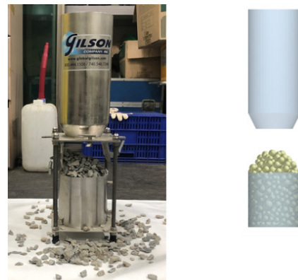
Fig. 2 Experiment and simulation of slump test(1 sphere model)
