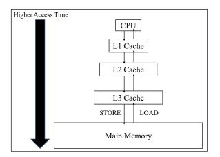
Fig. 1. Structure of a device with a multi-level cache (L1, L2, L3)
