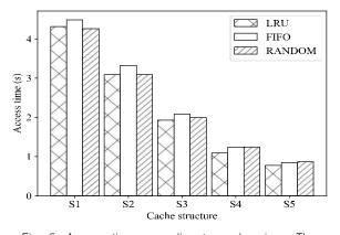
Fig. 5. Access time according to cache sizes. The cache structures are displayed below. S1: 16/250/500, S2: 32/500/1000, S3: 64/1000/2000, S4: 128/2000/4000,
