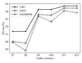
Fig. 6. Hit rate according to cache levels, with some structures including a fourth cache level. The cache structures are displayed below. S7: 128/2000/4000, S8: 128/4000, S9: 128/4000/8000, S10: 128/8000, S11: 128/2000/4000/12000, S12: 128/1000/2000/12000
