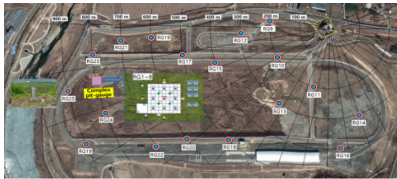
(a) Layout of EWRG (radius 1 km) and rain gauge network - Yeoncheon SOC center
