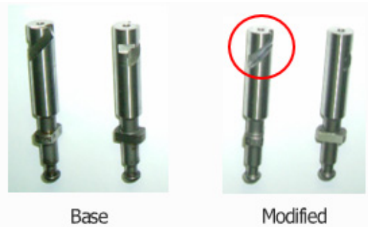
Fig. 3. Modified plunger of DME high pressure pump
