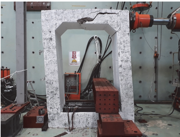
Fig. 14. Fragmentation of the specimen 2 by the test.
