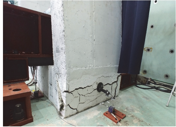
Fig. 15. Fragmentation of the bottom of specimen 1 wall.
