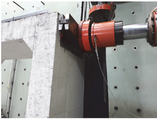
Fig. 10. The setting method for the loading bearing part.
