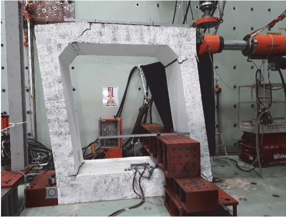
Fig. 13. Fragmentation of the specimen 1 by the test.
