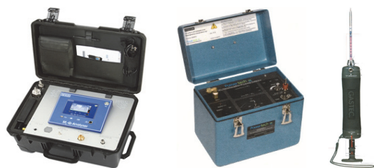
Fig. 1. Picture of on-site analytical equipment (from left, SF 6 Quality Analyzer [17], SF 6 DPD Analyzer [18], and Detection Tube [19]).
