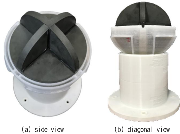
Fig. 8. Prototype of spherical flux concentration transmitter. (a) Side view of transmitter, (b) Diagonal view of transmitter.
