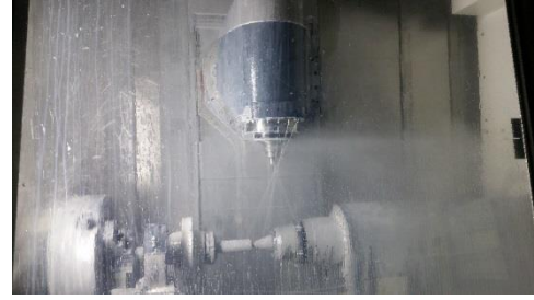
Fig. 8 Simultaneous 5-axis Turn-Mill machine
