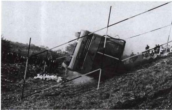
Fig. 1 Bus rollover test on 33.6° slope<sup>(7)</sup>
