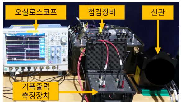
Fig. 11. Fuze and measurements setup
