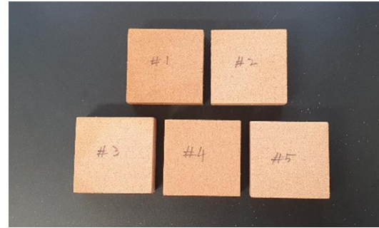
Fig. 9. PVC foam core specimens for density measurement.
