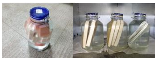
Fig. 14. PVC foam and sandwich structure specimens immersed in seawater.
