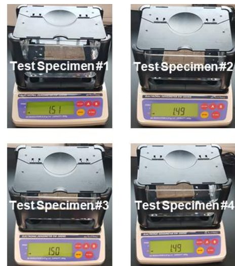
Fig. 5. Specific Gravity Measurement for GFRP Test Specimens using Hydrometer.
