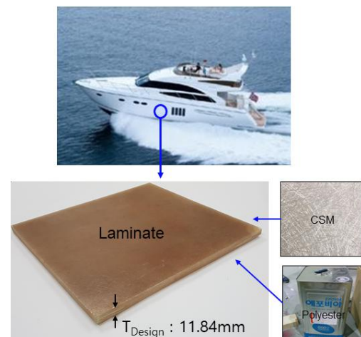
Fig. 2. GFRP Hull Plate of 16m Power Yacht.
