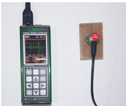
Fig. 6. Pulse-Echo Ultrasonic Testing (2.25 MHz Probe).
