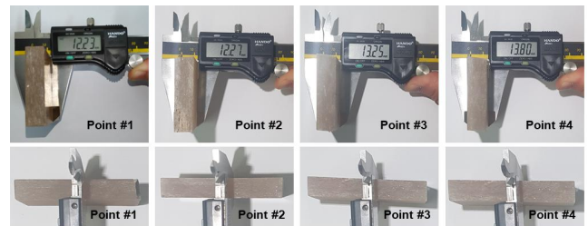
Fig. 4. Thickness Measurement of GFRP Test Specimens using Vernier calipers.
