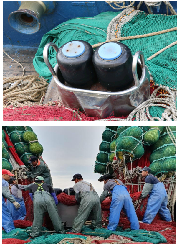
Fig. 5. Structure of ball roller and uses in the net hauling.
