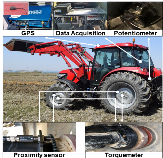
Fig. 1 Traction load measurement system for 78-kW class agricultural tractor
